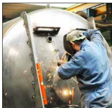
Manual welding of the accessories
