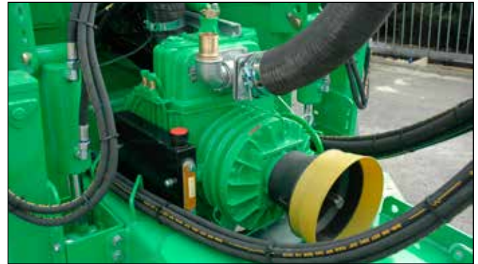
The JOSKIN Vacuumoil was especially developed to lubricate the pump vanes. A can is provided with each delivered vehicle.
