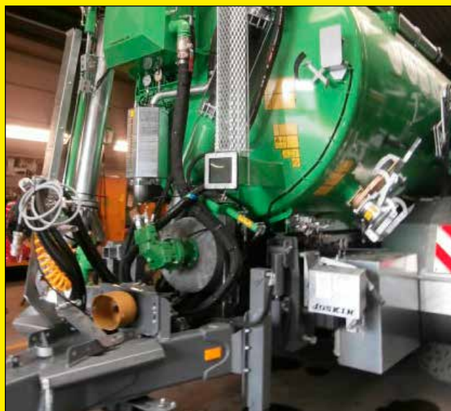
STORM with Power-Pack hydraulic drive
