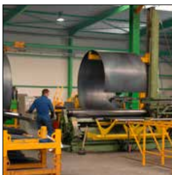
Bending the steel sheet (bending machine with digital control)
