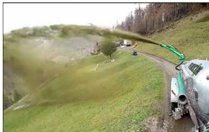
Vertical adjustment of spreading gun by hydraulic cylinder (in option)
