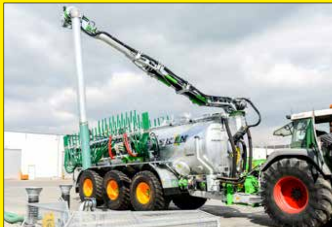
New dorsal boom with pivoting point at the front
