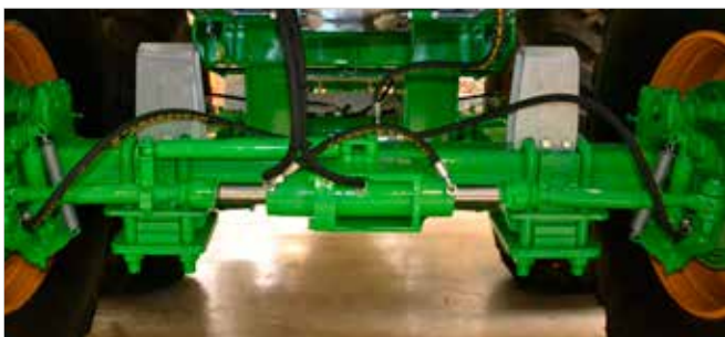
Free steering axle (50% steering)
