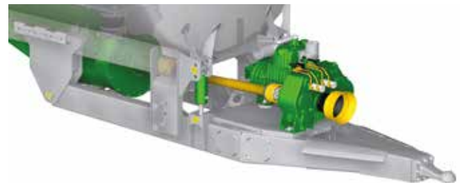
Mechanical drive of the 2 pumps through transmission box
