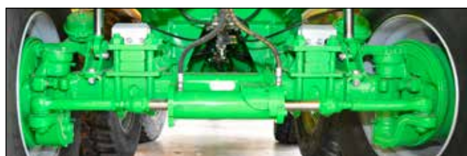
Self steering axle (100% steering)
